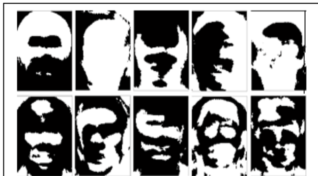
Fig. 3 shows the Eigen Faces of different faces obtained by using the PCA classifier. These Eigenfaces can be obtained by using the Equation (15).
